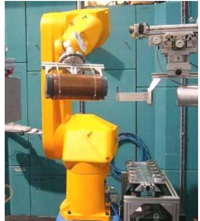
Robot as sample positioner for bulky samples (texture analysis)
