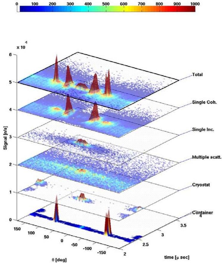
Figure J6 Virtual experiment data separating the scattering data into contributions from sample, sample container, cryostat, and multiple scattering. This cannot be done with a real experiment and could have huge future benefits.
