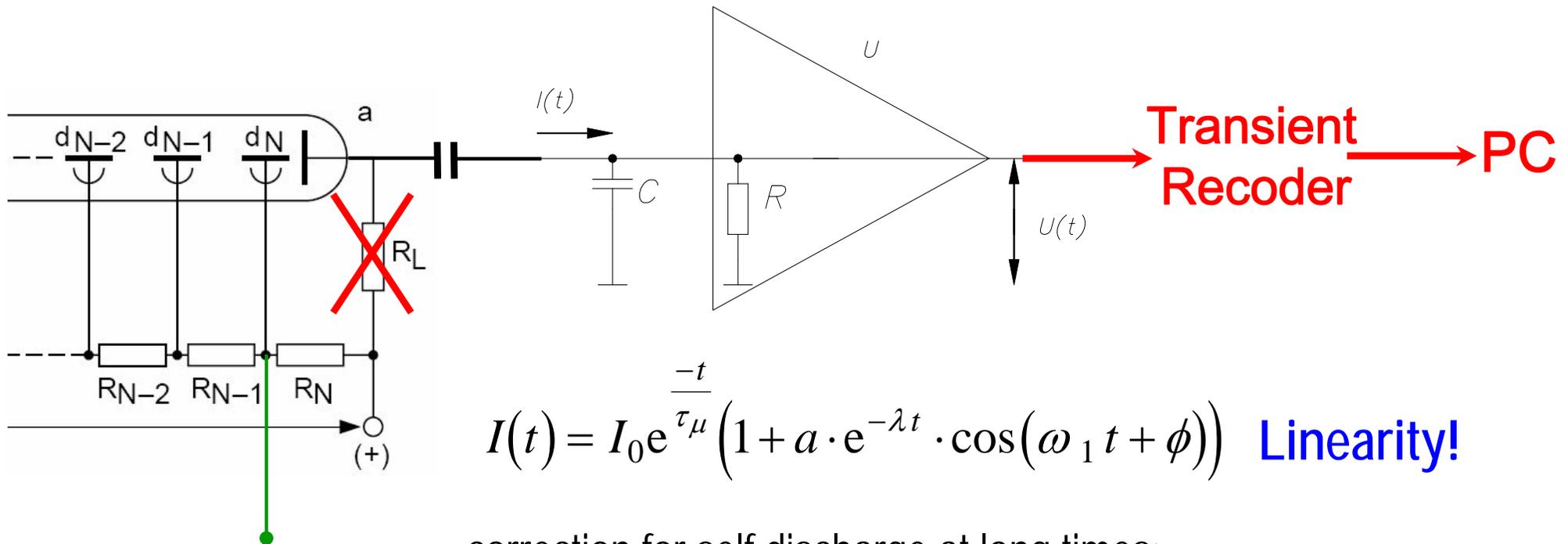
$$I(t) = I_0 e^{\frac{-t}{\tau_\mu}} \left( 1 + a \cdot e^{-\lambda t} \cdot \cos(\omega_1 t + \phi) \right) \quad \text{Linearity!}$$
