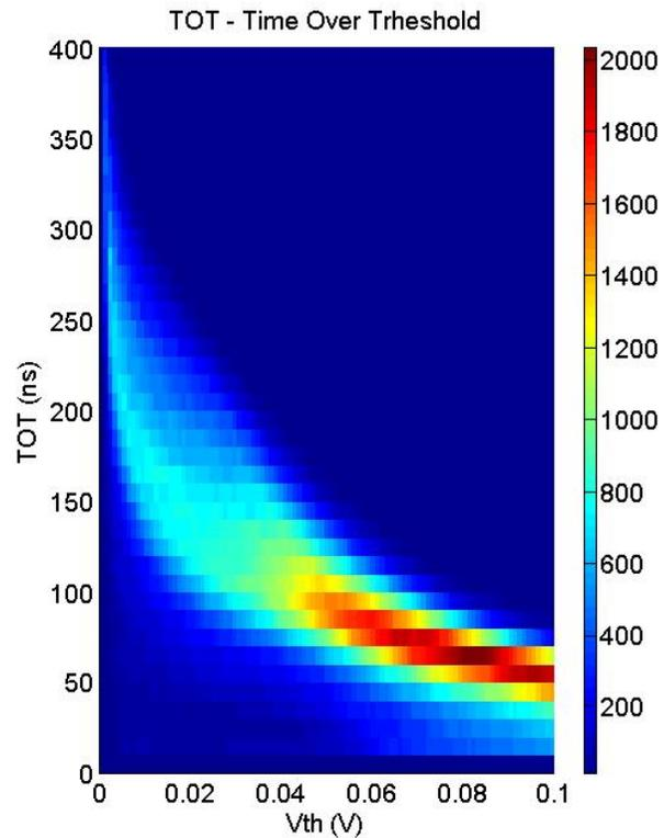
Total time over threshold for the PMT signals for a Threshold of  $V_{th}=5\text{mV}$
