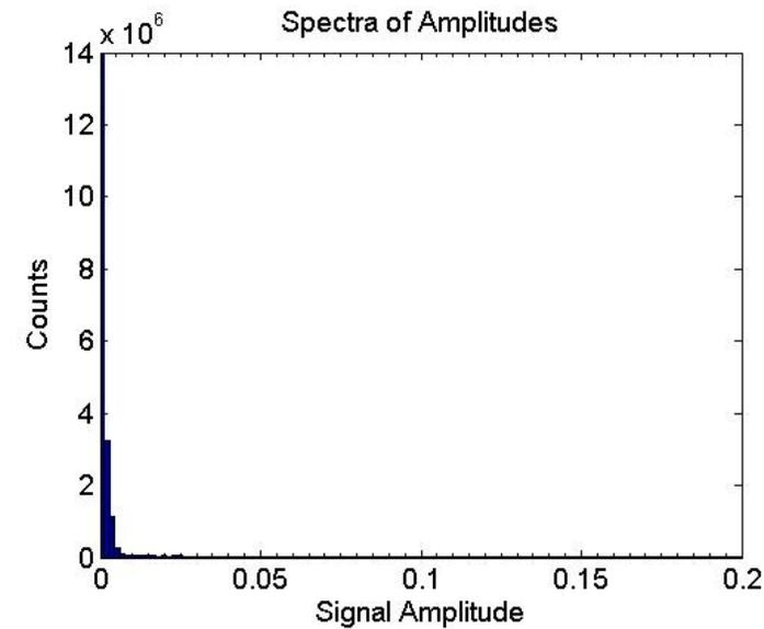
Noise level below 5mV  $\rightarrow$  Threshold=5mV
