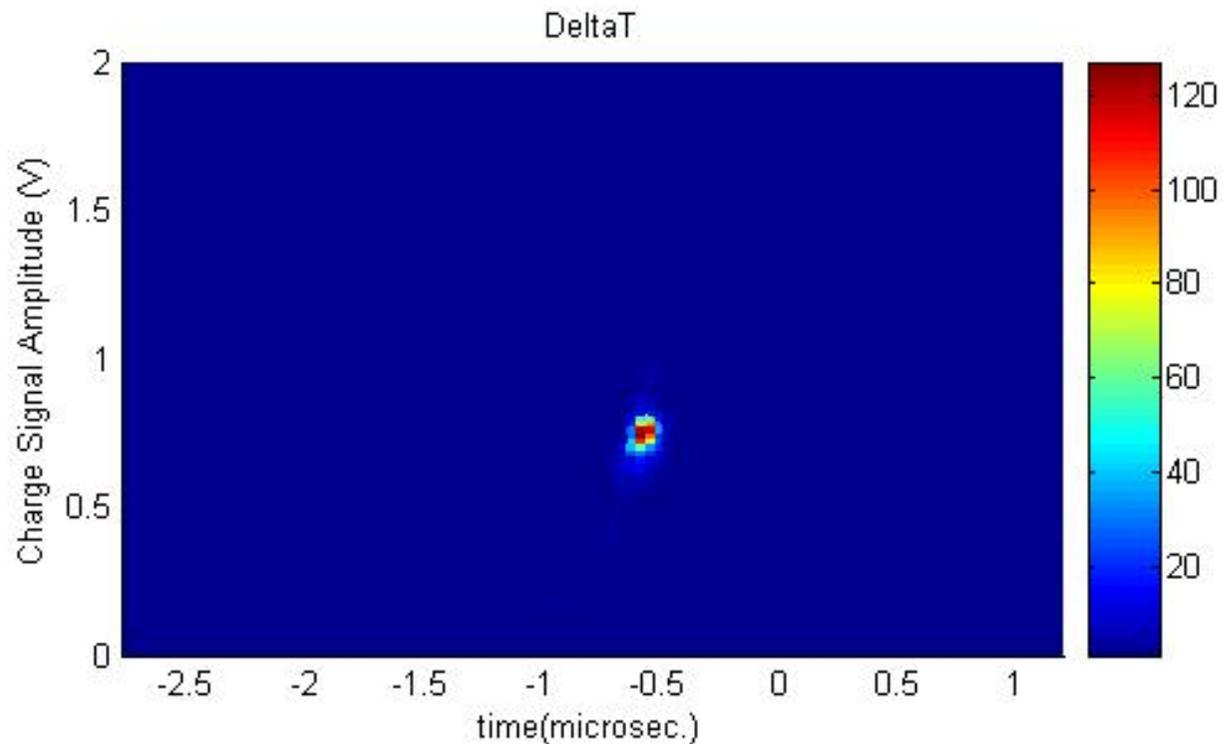
The maximum of the PMT signal is confined to a time window between  $-0.75\mu\text{s}$  and  $-0.25\mu\text{s}$  from the trigger
