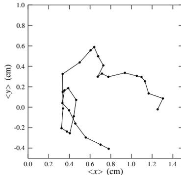
Figure 6: Simulation of the masking experiment Average values  $\langle x \rangle$  and  $\langle y \rangle$  plotted against each other showing the movement of the mean spot as the field is varied in increments of 0.1 T. Note that at  $B=0$  T,  $\langle x \rangle = 1.25$  cm and  $\langle y \rangle = -0.02$  cm.
