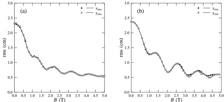
Figure 2: (a) Simulation results showing the rms beam-spot size oscillating with applied field for normal magnet operating conditions. (b) Measured results showing the rms beam-spot size oscillating with applied field for normal magnet operating conditions.
