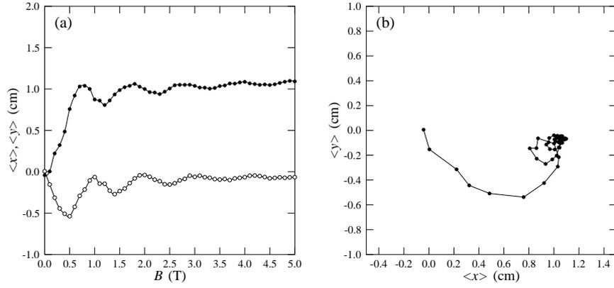
Figure 4: Simulation results for a tilting angle of 1 degree. (a) Average values  $\langle x \rangle$  and  $\langle y \rangle$  as a function of applied field. (b) Average values  $\langle x \rangle$  and  $\langle y \rangle$  plotted against each other showing the movement of the mean spot as the field is varied.
