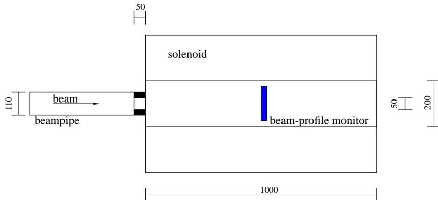
Figure 1: Apparatus used in the experiments. The muon beam travels up the evacuated beampipe, through a 50 mm diameter collimator (shown in black) and into the air filled magnet bore. The muons are detected by the beam-profile monitor (shown in blue). All measurements are given in millimetres.
