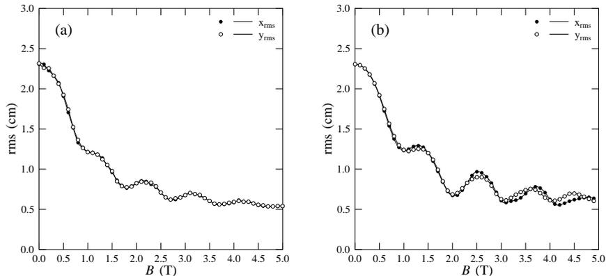
Figure 3: (a) Simulation of rms beam spot size in a field rotated by 1 degree. (b) Measurement of rms beam spot size in a field rotated by 1 degree
