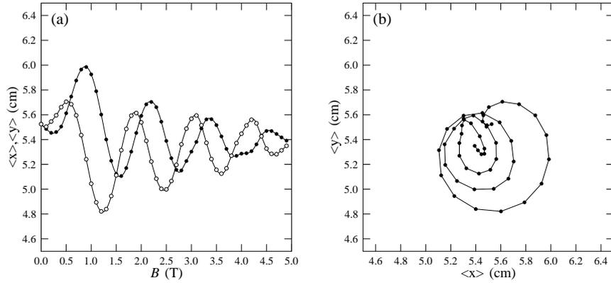
Figure 5: Measured results for a tilting angle of 1 degree. (a) Average values  $\langle x \rangle$  and  $\langle y \rangle$  as a function of applied field. (b) Average values  $\langle x \rangle$  and  $\langle y \rangle$  plotted against each other showing the movement of the mean spot as the field is varied.
